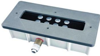
High performance LED Spot light. The most adaptable product on the marketplace. Ideal for stairs illumination, relax zones and beaches or small pool and spa bath. Waterproof sealing system. Outer thread 1 1/2" for installation on nozzle. 24 Vdc power supply. 5 m cable included. Power supply not included.
