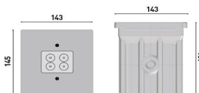
Small linear LED spotlight, suitable for residential swimming pools with PVC, tile or mosaic coating. Technopolymer niche with cable gland. Equipped with stainless steel flange gaskets and screws. Power supply not included. Made with IP68 waterproof connector integrated into the spotlight for connection to the cable to be customized. Suitable for application on prefabricated panels.
