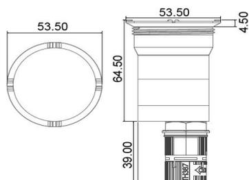
High performance LED Spot light. The most adaptable product on the marketplace. Ideal for stairs illumination, relax zones and beaches or small pool and spa bath. Waterproof sealing system. Outer thread 1 1/2" for installation on nozzle. 24 Vdc power supply. 5 m cable included. Power supply not included.
