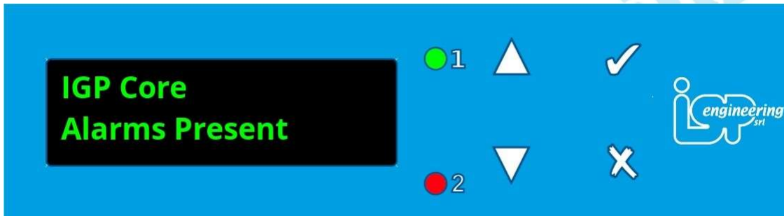
Figure 23: Pressing any button turns on the LCD, and the user will see IGP-Core HOME
