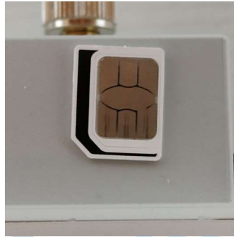
Figure 13: A uSIM Placed into a uSIM adapter
