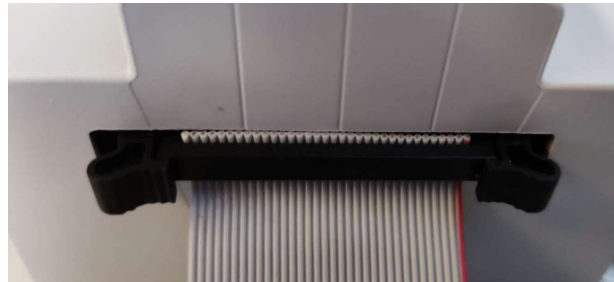
Figure 20: Expansion cable correctly inserted
