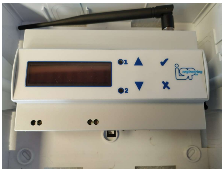
Figure 7: IGP-Core placed on a DIN rail
